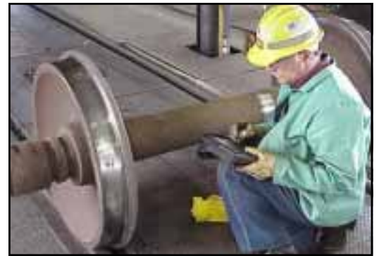
While performing a wheel inspection, a carman documents defects.
