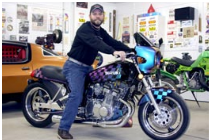
Machinist Brian Husa sits on his 1982 Suzuki GS, which he rebuilt with a salvaged GSXR 750 front end and a GSXR 1000 rear end.
